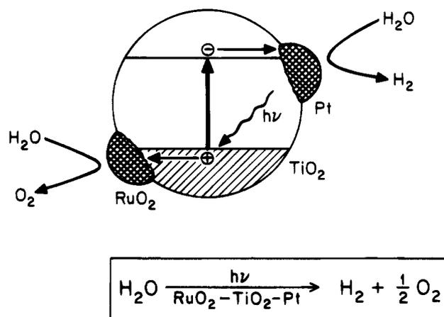
**Figure 3.7.** Photosplitting of water on composite catalyst.
