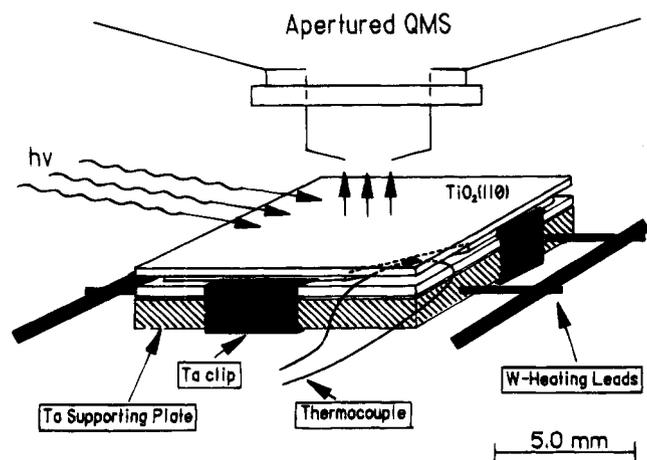
**Figure 3.10.** Design of crystal holder for photochemistry on TiO<sub>2</sub>(110) single crystal.
