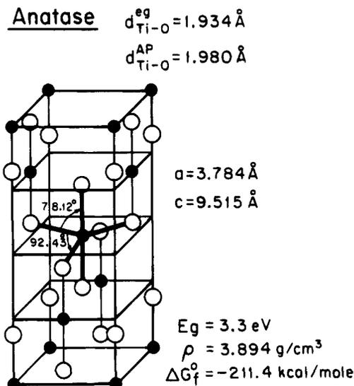
**Figure 3.1.** Structure of rutile and anatase TiO<sub>2</sub>.
