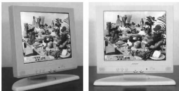
FIGURE 9.39. 17 inch AFLC display developed by DENSO CORP.
