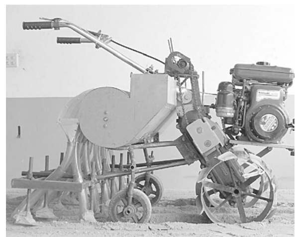
Figure 8 New mechanism at positions (1), (2) and (3) prototype 10-row garlic planter
