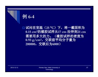
$$\sigma = \frac{\rho RT}{\overline{M_c}} \left( 1 - \frac{2\overline{M_c}}{\overline{M_n}} \right) (\lambda - \frac{1}{\lambda^2})$$
