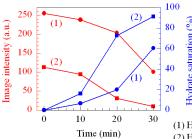
Saturation of THF hydrate formed in bulk as well in glass beads was estimated using the intensity of MRI images. MRI technique can be used to determine the spatial distribution of the hydrate phase and non-hydrate phase.
