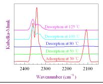
FT-IR spectra of  $\mathrm{Au/Al_2O_3}$  obtained during desorption in Ar at 50, 80, 100, and 125 °C separately after adsorption in 1%CO +  $10\%\mathrm{O_2} + \mathrm{Ar}$  (balance) at 30 °C.
