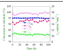
The tubular  $BaCo_{0.7}Fe_{0.2}$ - $Nbo_{0.1}O_{3-6}$  membrane reactor packed with Ni-based catalysts exhibited not only high activity but also good stability in hydrogen-enriched COG atmosphere.
