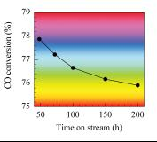
The catalytic performance of  $40\% Fe/60\% Ni/40 wt.\% Al_2O_3$  catalyst in different operation conditions has been studied. The results show that during the FTS a stable trend for this catalyst was observed.
