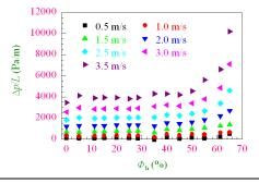
Pressure drops as a function of volume concentration of THF hydrate slurry.
