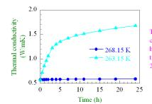
The effective thermal conductivity of methane hydrate sample versus time at 268.15 K and 263.15 K.
