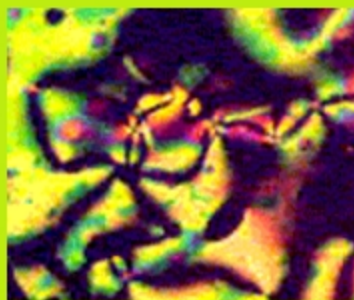
Figure 25 Nematic Schlieren texture. Schematic diagram of molecular (Han 2004)
