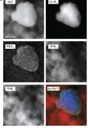
regation occurs during calcination to produce alloy nanoparticles having a Pd-rich shell surrounding a Au-rich core.
