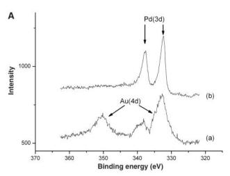
**Fig. 2.** (**A**) Au(4d) and Pd(3d) spectra for a 2.5 weight % Au–2.5 weight % Pd/TiO $_2$  catalyst after different heat treatments: (a) uncalcined or (b) calcined at 673 K in air. (**B**) Montage showing the ADF-STEM image of a bimetallic particle and the corresponding MSA-processed STEM-XEDS maps of the Au–M $_2$ , Pd–L $_{\alpha}$ , O–K $_{\alpha}$ , and Ti–K $_{\alpha}$  signals. Also shown is a reconstructed MSA-filtered Au–Pd–Ti composition map (Ti, red; Au, blue; and Pd, green).
